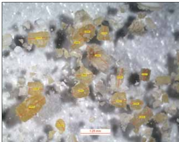
Figure 2. Particle size after grinding with simple food processor, Oster brand 600 W of power supply (M1).
